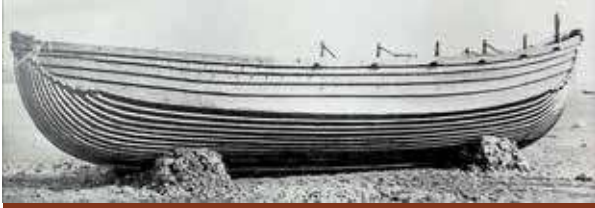
An Odishan Patia boat. partly of reserved clinker style, Image Courtesy - Aryan Books International
